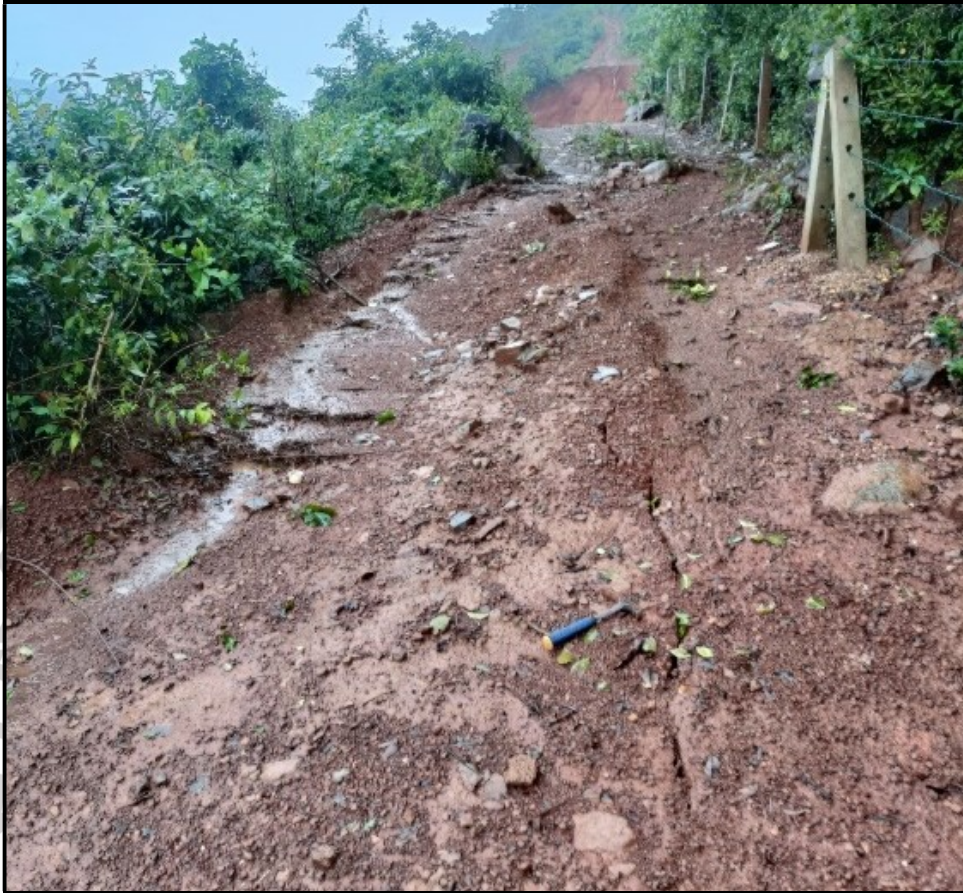
Fig. 1.11: Tension cracks at lower elevation of the left flank of the slide
